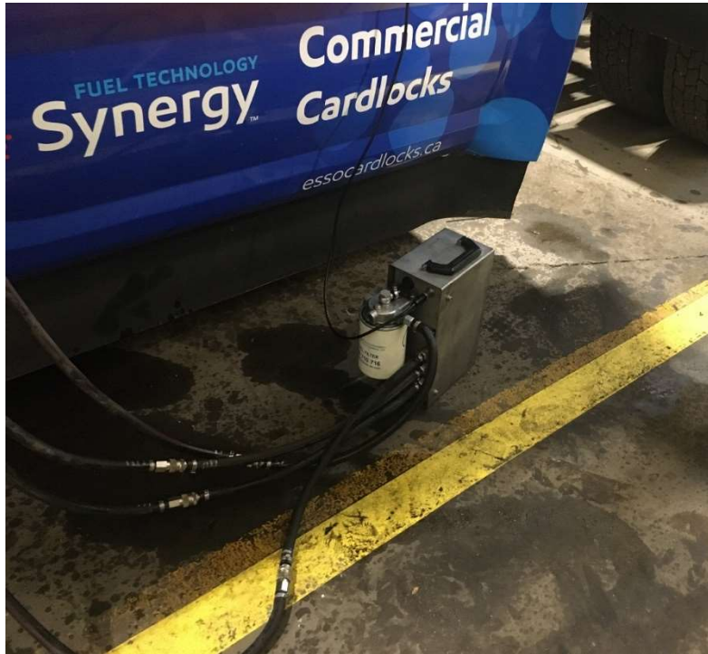
Figure D7: Air bleeding of AIC fuel flow meter
