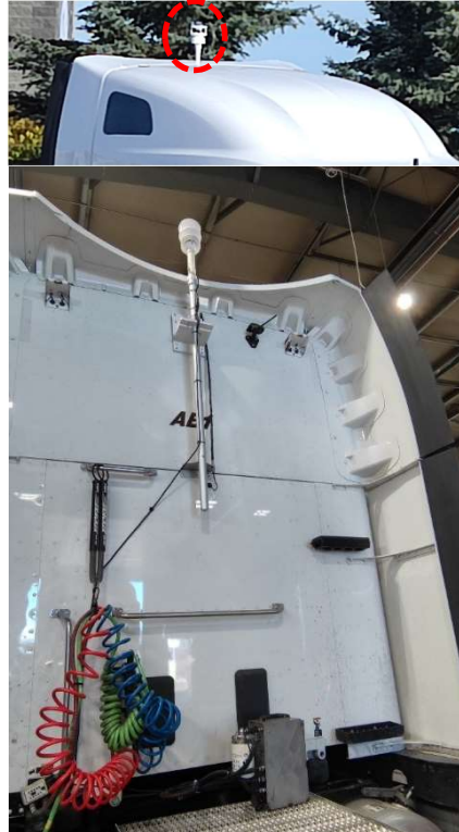
Figure 16: Vehicle-mount weather station
