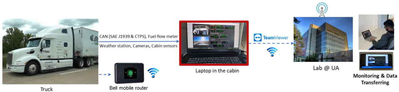
Figure 18: Data transferring and Remote Monitoring via Wi-Fi
