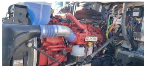
Figure 6: Cummins X15 engine in the Peterbilt 579 truck
