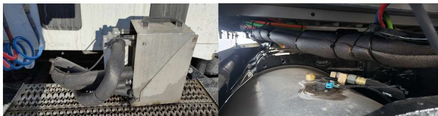
Figure 14: Insulation of hoses between the fuel flow meter and the engine
