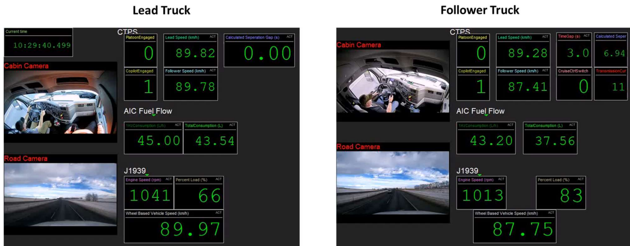
Figure 19: Graphical user interface (GUI) of the DAQ system during real time monitoring of truck operation
