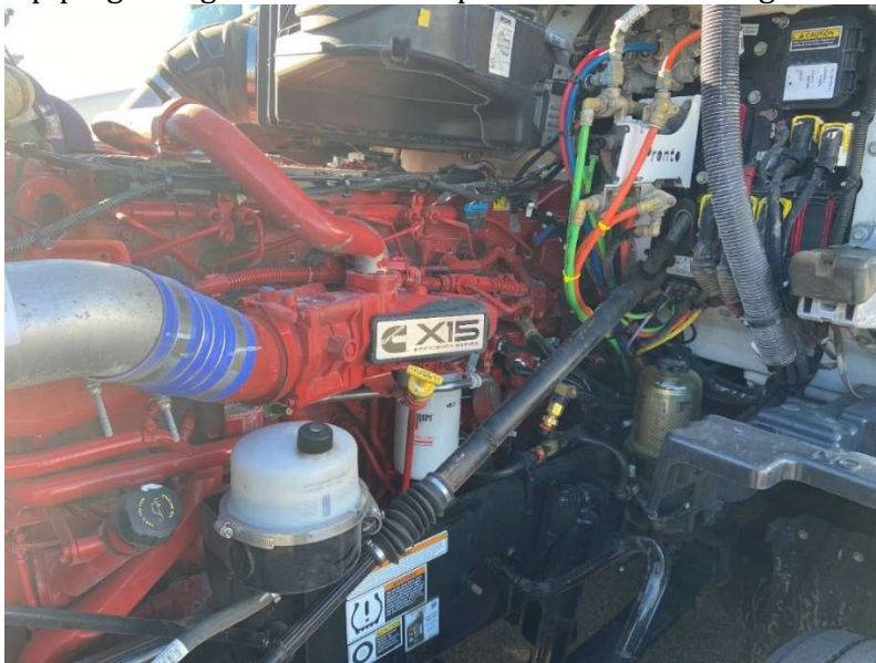
Figure D3: Fuel connections at driver side of engine, the connections were inspected as much as possible at AMTA yard
