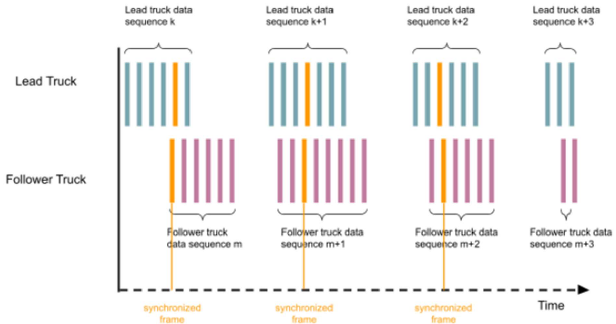
Figure 71. For data recording both trucks have arbitrary starting time and duration for the recorded data sequences, and that causes misalignment of the timestamps even if the GPS clocks for both trucks are assumed to be accurate. For scenario labeling the data frames for both trucks need to be presented in a synchronized manner with time difference between the two trucks as small as possible, as shown in the yellow synchronized frames as examples.
