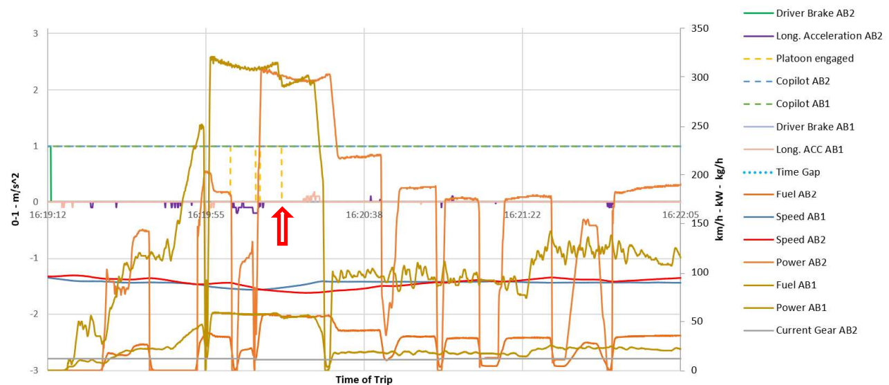
Figure 66: Event-based Copilot performance and its effect on the engine power oscillation
