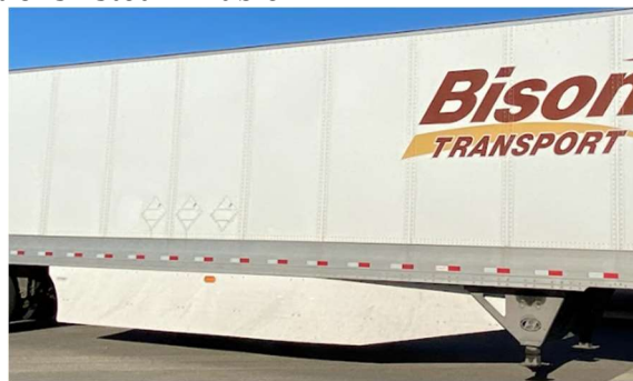
Figure 7: E-2330T side skirt model that was used in trailers for on-road trials in Alberta. The lower image is from transtex-llc.com.
