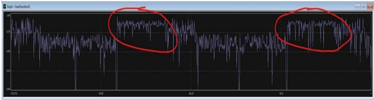
Figure 31: Gaze Direction Quality in a laboratory on a stationary table, when participants were asked to gaze at two fixed points.
